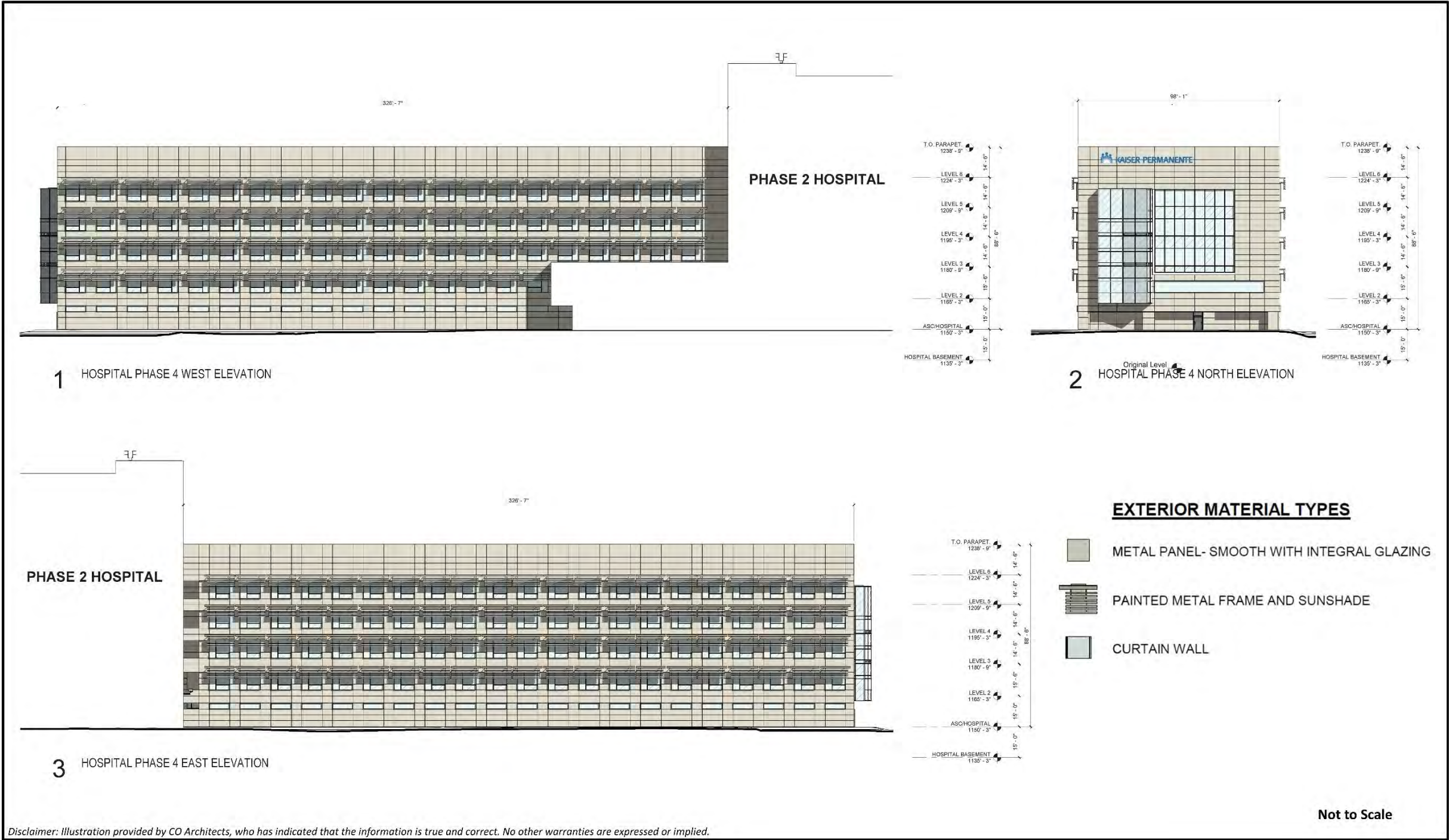
Figure 2.4-11 HOSPITAL ADDITION ELEVATIONS
