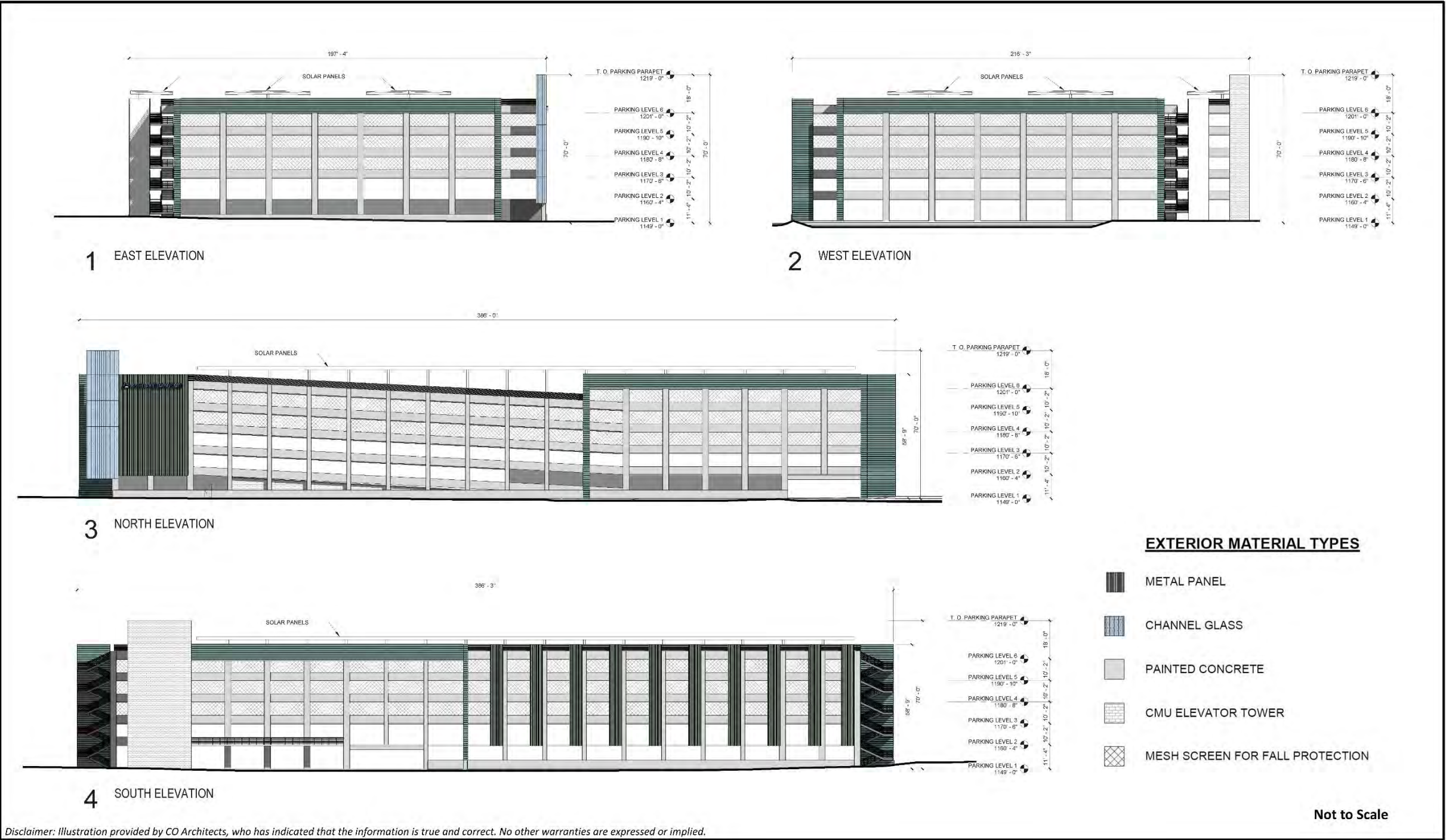
Figure 2.4-9 PARKING STRUCTURE ELEVATIONS
